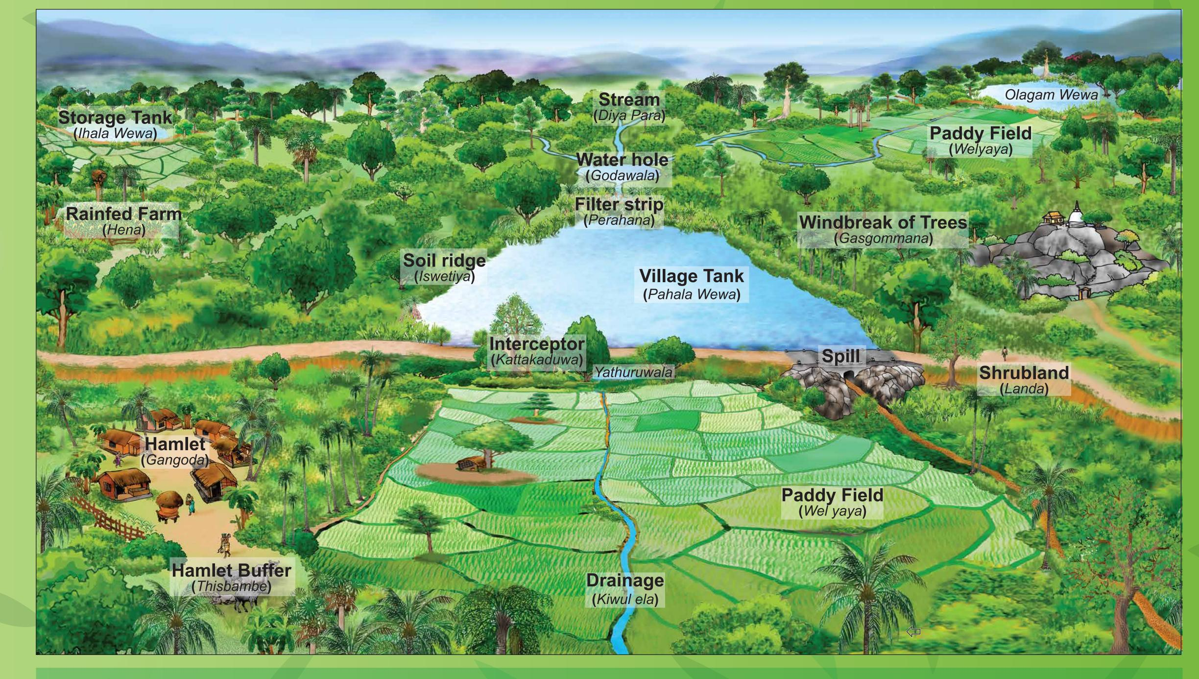
Layout of a small tank and its components
